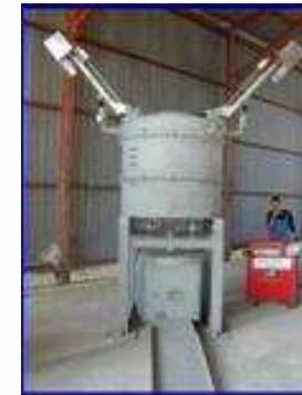
Plasma Reactor for ShipBoard Waste Treatment
